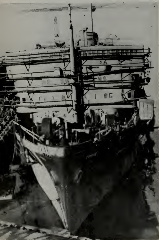
The Comber, one of a fleet of four 352-foot ocean-going, hopper type dredges being built by Ingalls for the Corps of Engineers, U. S. Army, recently was photographed in the wet docks of The Ingalls Shipbuilding Corporation's Pascagoula, Miss., yard, where she is outfitting.
